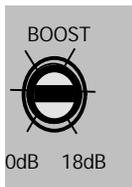
Turning the "BOOST" control clockwise increases the level of frequencies around 45Hz by up to 18dB when fully clockwise.
