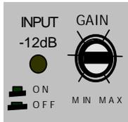
Adjust the input level for the marked channel(s) with a small screwdriver through the opening marked "GAIN". Turn clockwise to increase the level, counter clockwise to decrease. Amplifiers will run cooler and produce less system noise at lower level settings.
