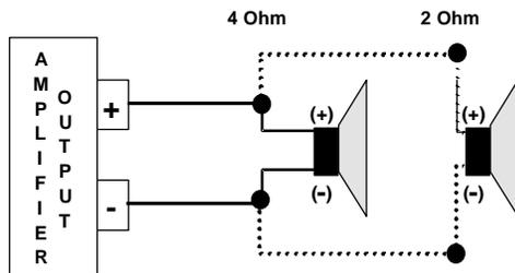
**SERIES-** Each additional speaker increases the load impedance for the amplifier. Impedances higher than 8 ohms are rarely used for car audio.
